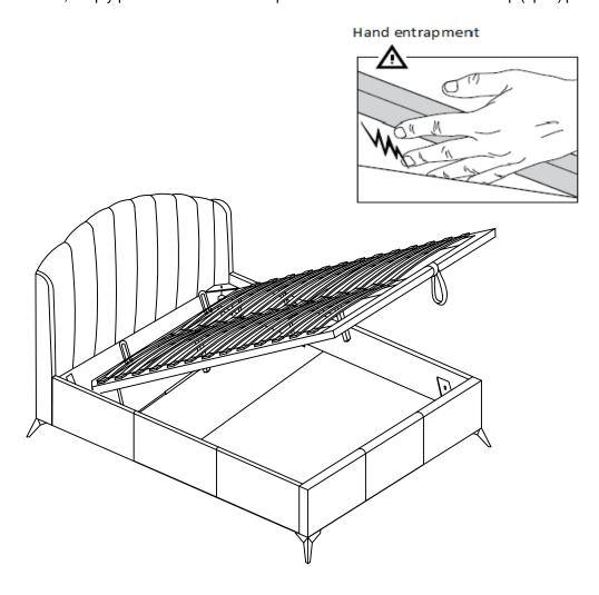
Lift with the strap and close with the strap. The strap should always be accessible. Take care not to lean over the bed when lifting, if the mattress is thin and light, the frame may rise quickly. The speed of closing will also depend on the weight of the mattress so always keep fingers well clear of the metal frame.
